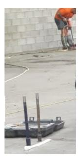
Unlike other cement cutting tools, core drill is hollow which allows it to carve out material from the drilled surface. In the case of applying Epoxy Coatings, Core drill can be beneficial to remove any cemented material on the surface of the concrete.
